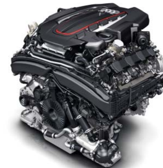
4.0 TFSI with Audi cylinder on demand technology
