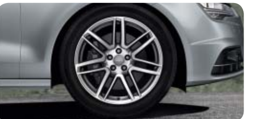
Audi Sport cast aluminium wheels in 7-twin-spoke design 3 size 9 J x 19 with 255/40 R 19 tyres 1
